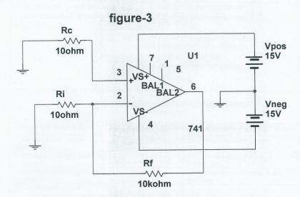
d) Estimate the input bias currents and input offset current for the Multisim 741 model given in figure-3 .
