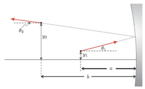
A light ray travels through a distance a, reflects from a curved mirror, and then travels through a distance b. The ABCD matrix has the following form:
