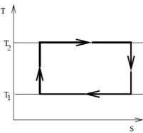
The figure shows the cycle's entropy-temperature diagram. Show that the efficiency of the cycle is
