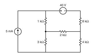
Calculate all of the unknown voltages and currents in the above circuit, using either the node-voltage, mesh-current, or superposition method (your choice.) Mark your answers directly on a copy of the circuit. In all cases, label the *actual* direction of current flow and the true polarity of the voltages (i.e., none of your indicated quantities should be negative.)
