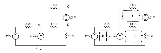
(a) Use the node-voltage method to derive a set of linear equations that can be used to solve for the two unknown node voltages  $v_A$  and  $v_B$  in the above figure. Collect your equations into a matrix equation of the form:  $\mathbf{A}\mathbf{x} = \mathbf{b}$  where
