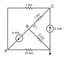
(a) Use the node-voltage method to derive a set of linear equations that could be used to solve for the unknown node voltages  $v_A$ ,  $v_B$  and  $v_C$  in the above figure.
