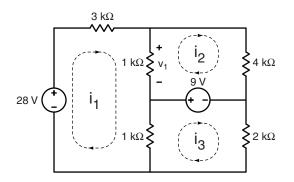
(a) Use the mesh-current method to derive a set of linear equations that could be used to solve for the unknown mesh-currents  $i_1$ ,  $i_2$  and  $i_3$  in the above figure. Collect your equations into a matrix equation of the form:  $\mathbf{A}\mathbf{x} = \mathbf{b}$  where
