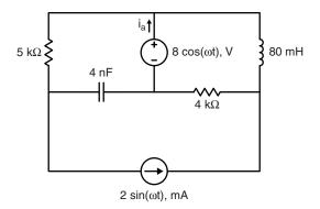
Solve this circuit using either the node-voltage or mesh-current method. Then answer the following questions:
