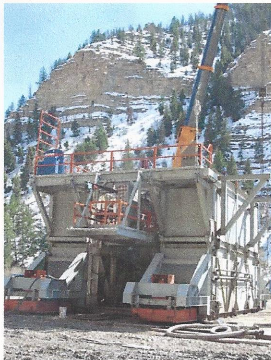
Photo 1: Walking rigs are large land-based rigs used on locations where numerous wells are drilled in a small area.
