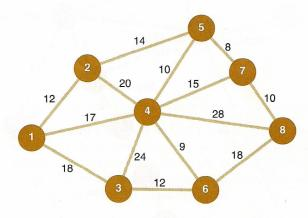
Determine the shortest route a concrete truck would take from the plant at node 1 to node 8 and the total distance for this route, using the shortest route method.
