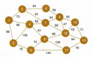
Determine the shortest path from node 1 in north Georgia to node 13 in Virginia and indicate the total mileage of the trail.
