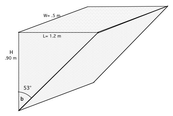
Prism shown submerged in liquid with horizontal upper surface at depth B. Line of sight perpendicular to face.
