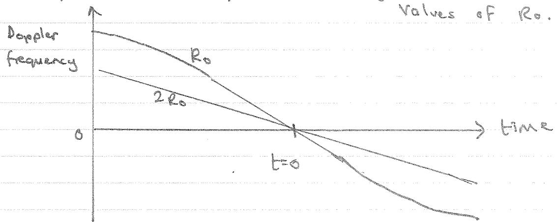
Note that for  $\theta_0 = 90^\circ$ , at  $t=0$  the vector to  $P$  is perpendicular to the velocity vector, hence the Doppler is zero.
