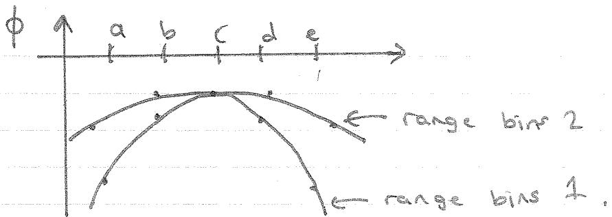
We note that the next range bin, say 2, corresponding to  $A_2, B_2, \dots$  has a different phase compensation curve given its longer range & lower Doppler.
