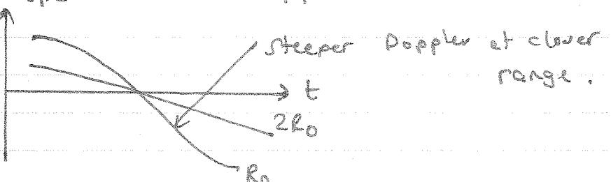
In broadside SAR,  $r_0$  is the slant range at the point of closest approach C. Because different filters are req<sup>2</sup> for different ranges, one could argue the the use of Doppler filtering to resolve range. However, a much better resolution is obtained conventionally in the delay domain.
