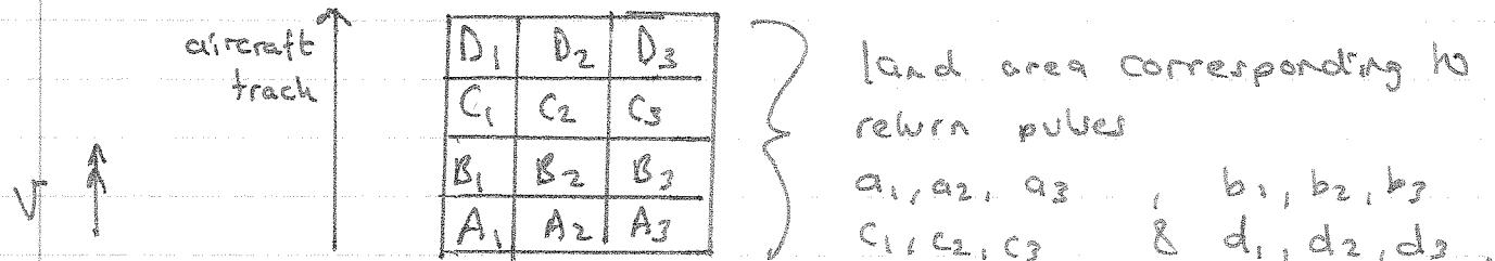
Pulse  $T_b$  is emitted when the aircraft is in line with row B. Unfortunately, the return at bin  $b_1$  does not come from area element B, only.
