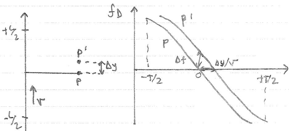
For SAR with a  $90^\circ$  squint angle, the Doppler history of returns from  $P$  &  $P'$  are two parallel, descending, nearly straight lines. The frequency separation between the two is  $\sim$  constant.
