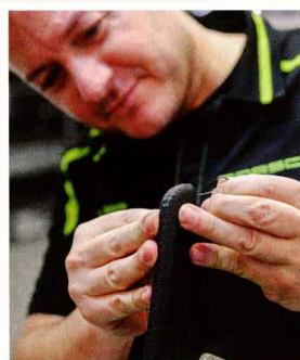
It takes around 40 minutes to hand-stitch each pair of sun visors for a 918 Spyder
