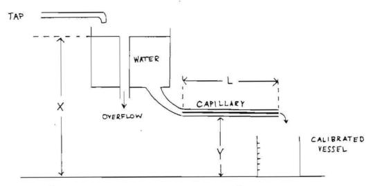
THEORY: The rate of flow of a liquid (cm<sup>3</sup>/s) through a capillary is directly proportional to the pressure gradient across the capillary:
