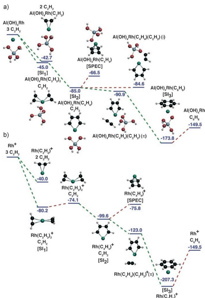
Figure 5. Theoretical potential-energy surfaces characterizing the triplet potential energy surface for acetylene cyclotrimerization catalysis by a) supported  $\text{Rh}^+$  ion modeled as  $\text{Al}(\text{OH})_4\text{Rh}$  and b) gas-phase  $\text{Rh}^+$  ion. Energies are given in  $\text{kcal mol}^{-1}$ . The triplet surfaces are shown for comparison with the very similar singlet surfaces shown in Figure 4.
